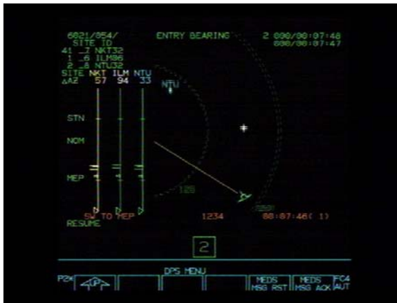
ECAL Entry to Cherry Point (NKT) with High \Delta Az - MM602 Post Nz Hold
